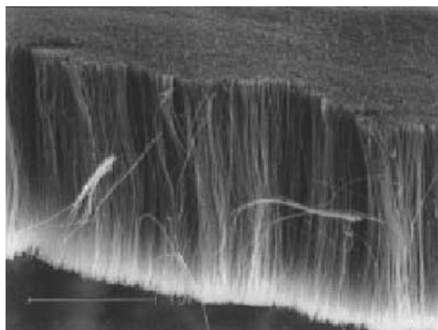
Figure 9. A typical SEM image of the aligned carbon nanotube film prepared by pyrolysis of FePc. The misalignment seen for some of the nanotubes at the edge was caused by the peeling action used in the SEM sample preparation. [58]
