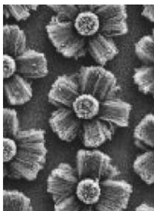
Figure 22. Multidimensional aligned carbon nanotubes grown out from \text{SiO}_2 polygons prepatterned on a Si substrate. [108]
